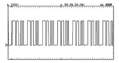
We can see the triggered "glitch" at the left of this small fraction of the waveform. We scrolled using the Agilent 54645A's MegaZoom technology that allows us to zoom and pan through the data even after it has been acquired, but were unable to see another glitch even though we captured over 1000 cycles of the pulse pattern. This proved the glitch was indeed infrequent, and showed the value of the "time-qualified trigger" function.
