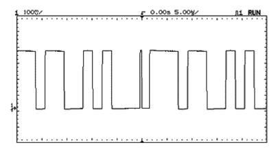
With the time reference of the screen set to "center", the glitch appeared as predicted at the center of the screen. Although the glitch occurs only once every few thousand cycles, it was easy to see it on the digitized screen. We then expanded it to get a closer look at the "glitch":
